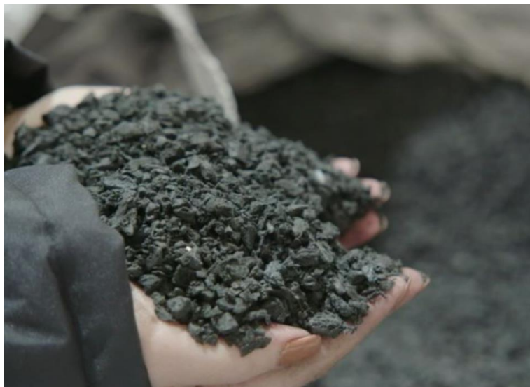
Figure 7: Thousands of plastic bags and old printer cartridges turned into road additive
